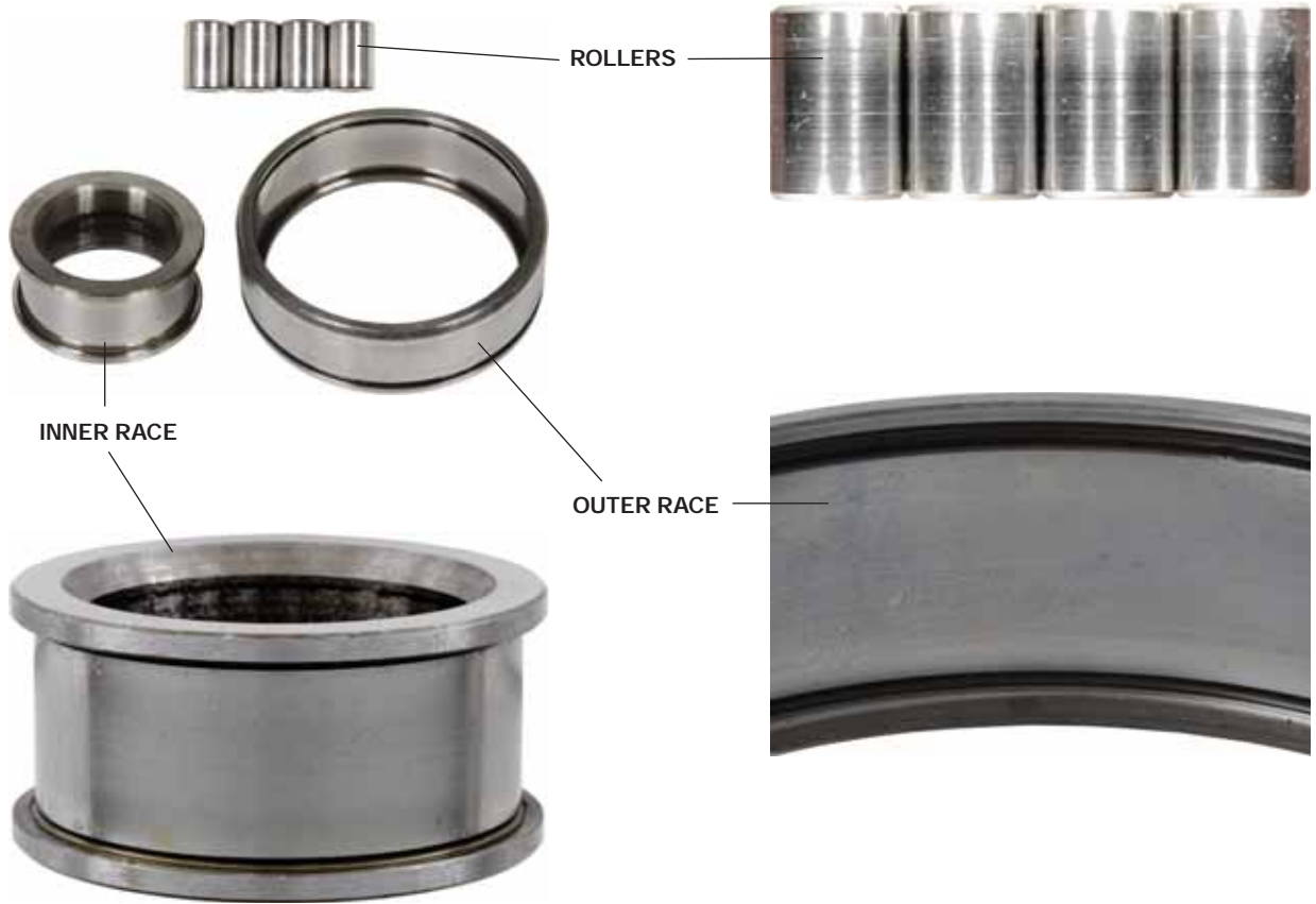
Upper Right Front Countershaft Bearing Merit Ratings
