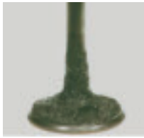
Intake valve before P.i. treatment.
