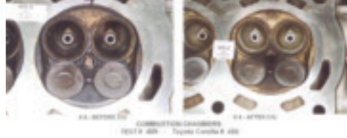
Combustion chamber before P.i. treatment. Combustion chamber after P.i. treatment.
