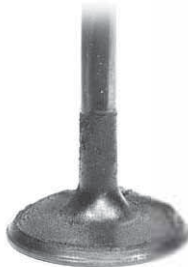
Intake Valve after P.i. Treatment
