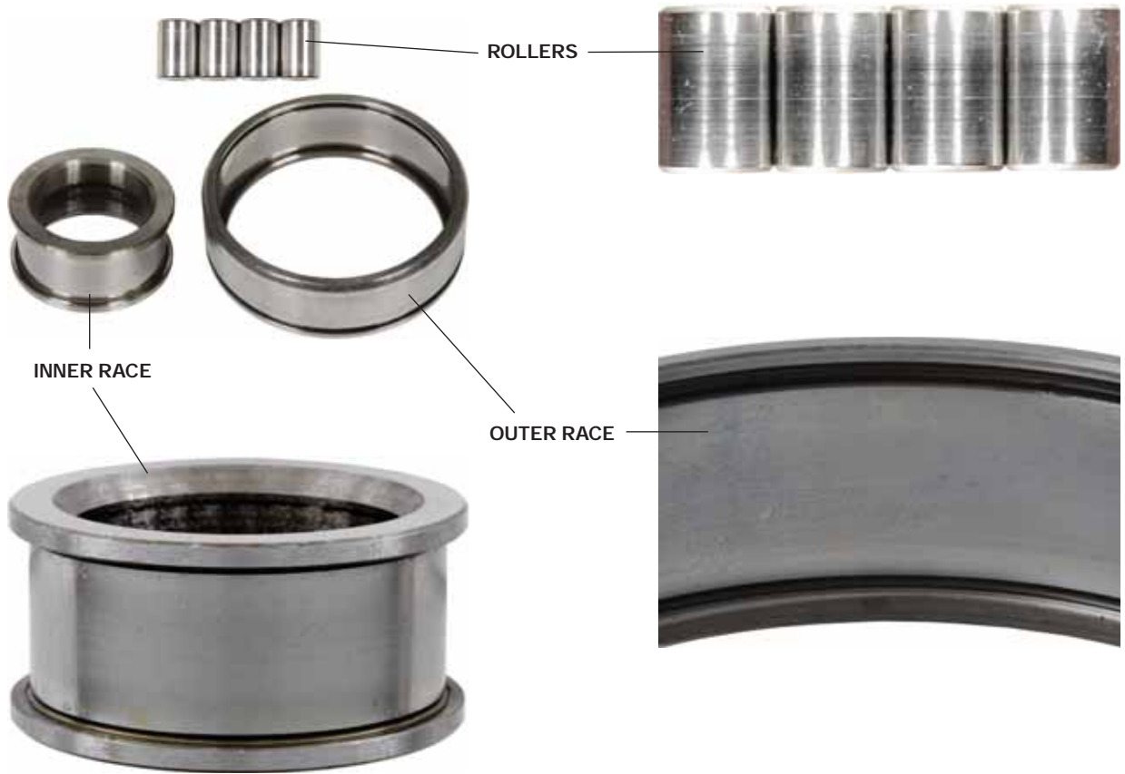
Upper Right Front Countershaft Bearing Merit Ratings
