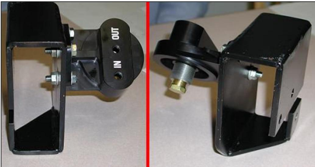
In these images you can see that the corners were created when the inside corners touched and were clamped in place on spacer blocks and then welded.
