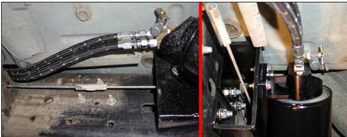
The cap you see was created by hand screwing a brass or steel 1/4" close nipple into a 3/8" - 1/4" pipe reducer. You will need to hold it in a vise to drill the close nipple out enough to fit over the spigot of the sample valve. I cleaned both with brake cleaner to remove all oil, then wiped with a tinning solder paste and heated till tinned. The nipple was cut off flush
