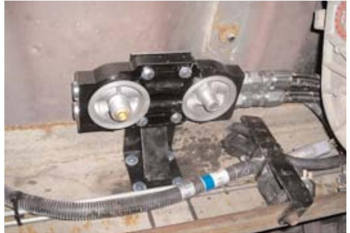
Completed installation with EaBP100 and EaO26 installed.
