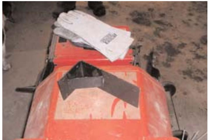
The mounting bracket that was fabricated for this installation.
