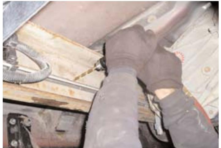
Drilling holes in the frame to install the mounting bracket. The holes were center-punched using a transfer punch to get the exact locations.
