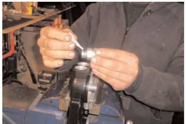
Applying the AMSOIL-supplied thread sealant to the valve block adapters.
