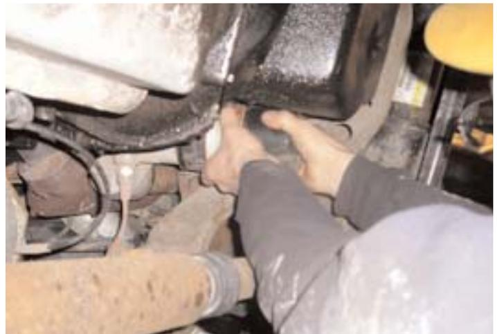
Removing the old full-flow filter.
