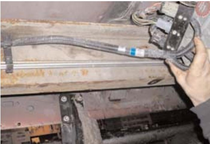
Removing the bracket that holds the transfer case clutch connectors to make space for the BMK26 mount. The bracket was re-installed later.
