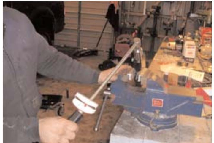
Installing the valve block adapters and plugs to the proper torque.
