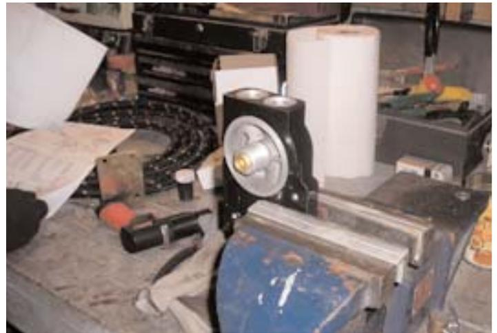
Loctite thread locker was used on the grade-8 bolts and nuts used to bolt the bracket to the frame.
