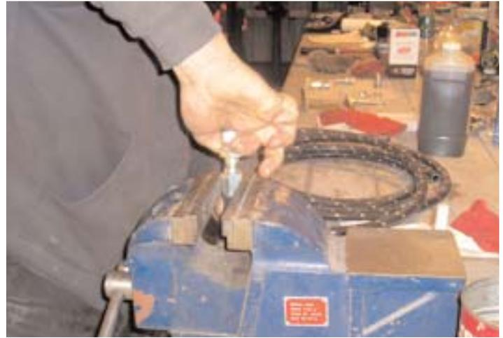
Installing the hose-end fittings. Note that the tapered adapter fitting in the above photo was lightly oiled so that it would install and fit properly in the hose during the tightening procedure.
