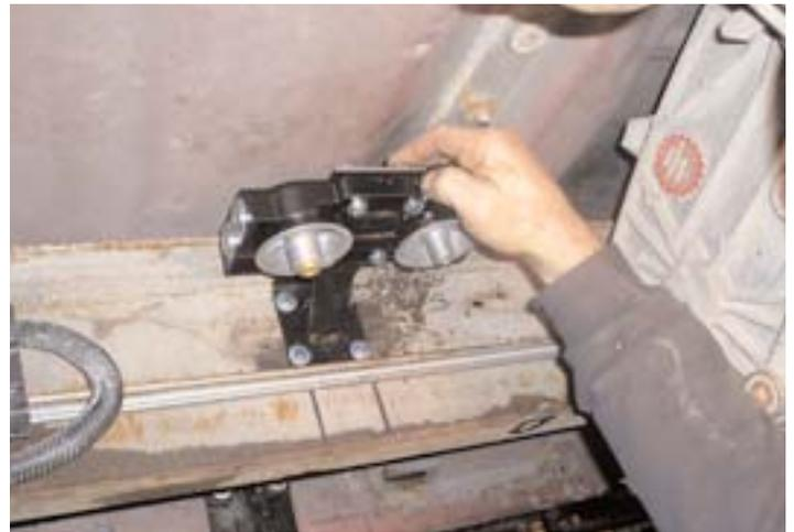
Bolting the valve block to the mounting bracket.
