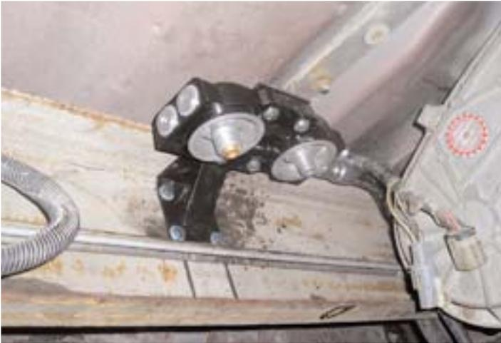
Final installation of the valve block with both hoses installed.
