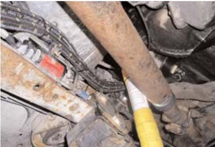
Hose route on the driver's side inner frame rail. It was zip-tied and secured so that it cannot interfere with the front driveshaft. There must be a small amount of slack left in the hose to allow for engine roll.
