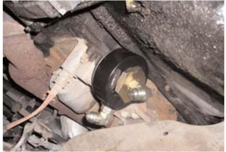
Installed engine adapter positioned so that the hose would be routed smoothly to the driver's side frame rail and away from the front driveshaft.
