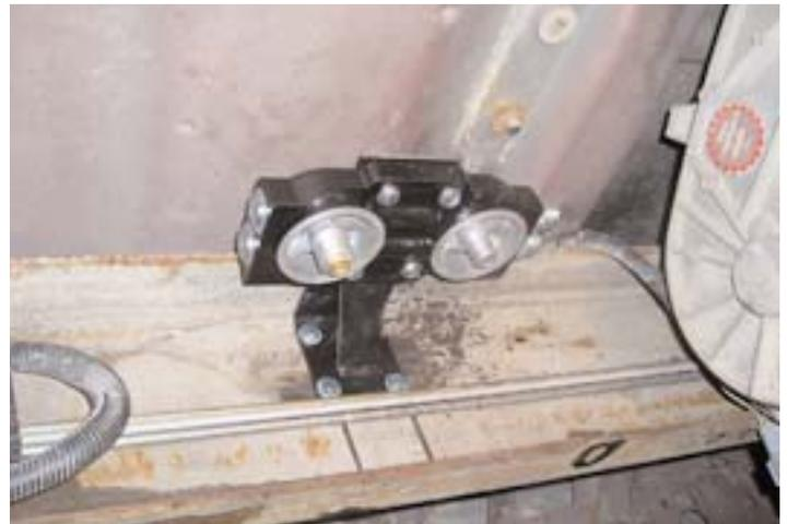
Bolting the valve block to the mounting bracket, continued. Note that, although the nuts supplied with the kits have a self-locking feature, Loctite was used as an extra measure of safety from vibration.
