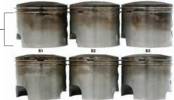
Starboard side of engine using Evinrude XD100
