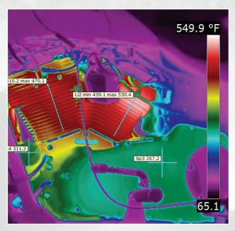
As temperatures climbed to more than 500°F in the cylinders, an infrared camera revealed the red-hot conditions that assaulted the engine components and oil.
