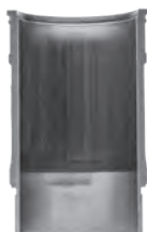
Severely Scuffed Liner
