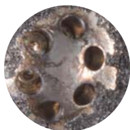
Injector after one P.i. treatment.
