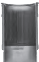
Severely Scuffed Liner
