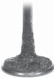
Intake valve before P.i. treatment.
