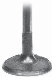
Intake valve after P.i. treatment.
