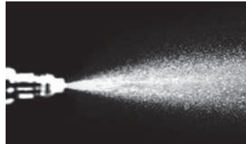
Injector spray pattern after P.i. treatment.
