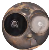
Cylinder head after one P.i. treatment.
